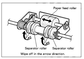
5 Following the same procedure as in step 4, use the accessory roller cleaning paper to wipe the surfaces of the retard rollers all the way around them proceeding from one end to the other in the directions of the arrows shown in the diagram to the right.
